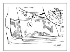
7.4 Headlight retaining bolt (A), and retaining spring arrangement (B)
